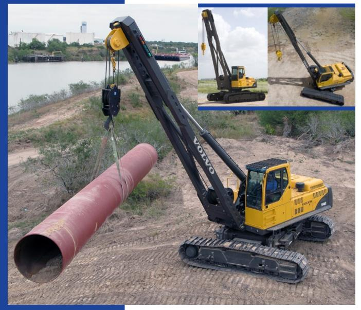
Volvo Pipelayers are purpose designed and built to meet the rugged application requirements of the pipeline industry. Their design provides state-of-the-art safety and lifting technology in a 360-degree working platform. Versatility to be converted to a conventional excavator further increases their potential for utilization.
