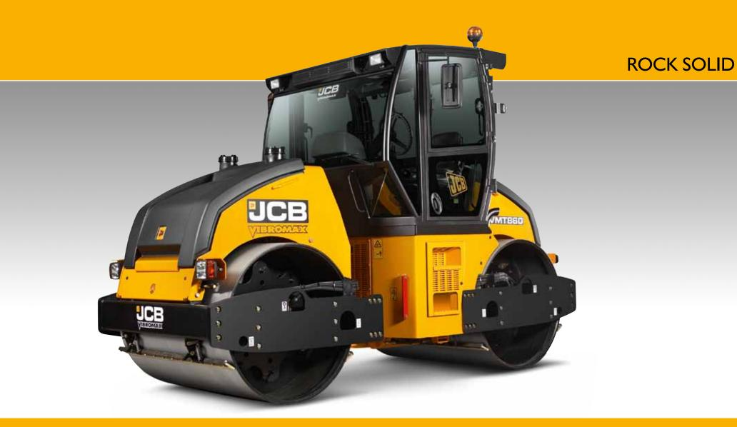
The JCB Vibromax range of vibratory tandem rollers is renowned for its excellent combination of static weight, centrifugal force and amplitude. The new VMT860 is no exception. Quite simply, the VMT860 sets the bar, and sets it very high, for heavy asphalt and soil compaction.
