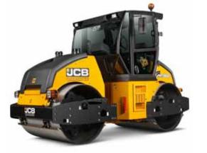
Optimal static weight, high centrifugal force and amplitude. Together, these three essential elements make for extremely high compaction performance on asphalt base, binder and wearing courses. The excentric system creating the centrifugal force is unique as a result of its simplistic single piece eccentric shaft with over turning weights, which guarantees market-leading values for t/h (asphalt) and m<sup>3</sup>/h (soil), minimising the cost of operation.
