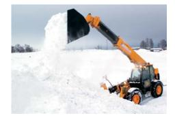
JCB Loadalls are also designed to give you the clearest view, essential in bad weather. So, low-mounted booms ensure good visibility across the machine, a massive glass area provides unsurpassed all-round visibility, and front, rear and roof wipers clear snow efficiently making sure the operator's view remains unobscured.
