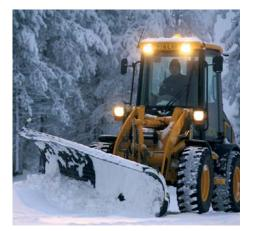
Every model also features a choice of torque proportioning or limited slip differential axles. These deliver exceptionally powerful tractive effort, for minimum sliding while pushing snow. The axles also house the service brakes: oil-immersed for minimum wear, self-adjusting for constant efficiency.
