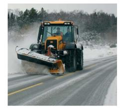
The 248hp, 8.3-litre engine JCB 8250 is our latest Fastrac model. At the heart of this unique machine is the V-Tronic continuously variable transmission (CVT). This increases operational potential by giving you: uninterrupted acceleration and deceleration; a number of different operating modes; and clutchless direction changes for smoother operation.
