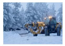
With capacities of 2 to 2.7 tonnes and lift heights from 4 to 5.6 metres, JCB compact Loadalls are perfect for confined sites. All are fitted with Tier II compliant JCB diesel engines for ease of operation and excellent pushing power, particularly at low speeds.
