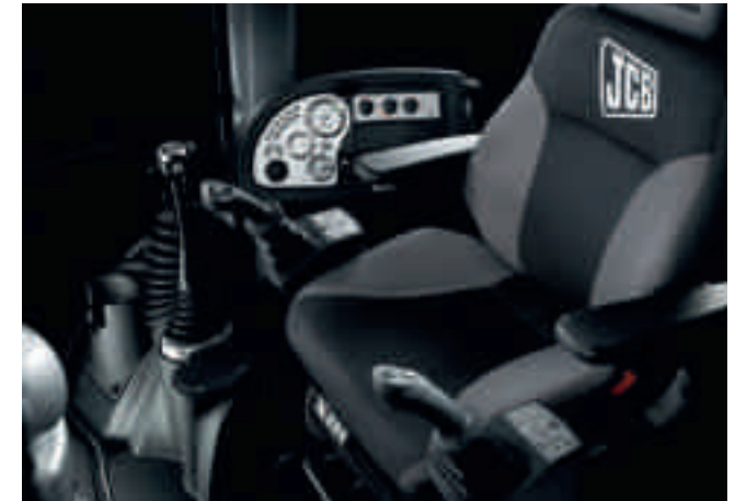
Precision Control system with integrated, seat-mounted controls
