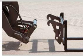
Volvo hydraulic quick coupler for fast attachment changes.
