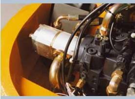
Separate working and steering hydraulic pumps provide fast cycle times without losing power or control.
