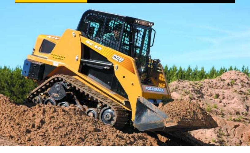
The ASV RC-60 is a mid-sized Rubber Track Loader with exceptional power, performance and an outstanding list of leading-edge features. Included is ASV's RTSS II<sup>™</sup> rubber track undercarriage with suspension. This advanced system gives you maximum traction and stability for working more productively in a wider range of conditions. Ground pressure under the 15 inch wide rubber tracks is only 3.5 psi.
