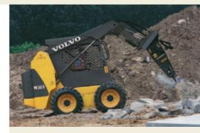
Break it up with the hydraulic hammer.
