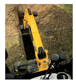
The 8014 may be small but that doesn't mean it isn't tough. Key to this is the brand new tubular boom. Stronger than a flat design, it is light yet rigid for outstanding durability. But because it's hollow, you can also run all the dig-end hoses through it, protecting them from site damage.
