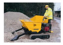
There's also an optional self-loading shovel, which eliminates the need for the operator to manually fill the machine, and low ground bearing pressure means you can carry on working in even the wettest ground conditions.
