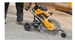
A 66.7cc, two-stroke engine provides 3.0kW of power for the most productive construction work and it's quick and easy to adjust the belt tension to ensure maximum transfer of this power to the disc for the most efficient cutting.
