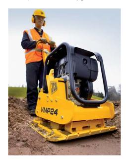
they can be fitted with rubberised plates for the compaction of paving stones and block paving, and used without the rubberised plate for sand compaction before laying block paving.
