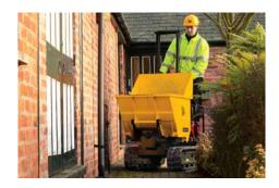
We've recently expanded the range to include a new Hi-Tip model. This combines the class-leading benefits of our other Dumpsters with the capability to tip to a height of 1,650mm, so it's perfect for unloading building and landscaping materials, earth and debris into a high-sided skip or drop-sided truck. But despite the additional lifting height, the Hi-Tip is no wider than standard models so it can still get through a doorway or garden gate.
