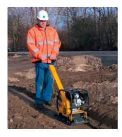
durability. With weights ranging from 68kg to 130kg and with working widths of 350mm to 500mm, there are four popular models to choose from.
