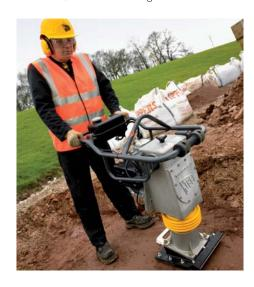
Powered by four-stroke petrol engines, the two models offer operating weights of 60kg and 73kg respectively. Both feature a strong and sturdy, low-maintenance design that results in longer
