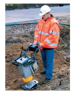
working hours for higher productivity. They also have a low centre of gravity with a four-column guide and stable function, guaranteeing high reliability for continuous, fault-free working.
