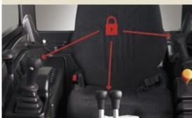
· Controls lock when the safety strut is raised.
