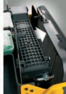
· Tilting cooler/radiator access for easy cleaning.
